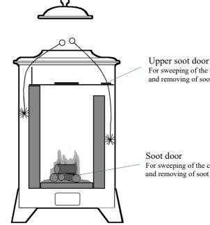
For sweeping of the channels and removing of soot and ash.
